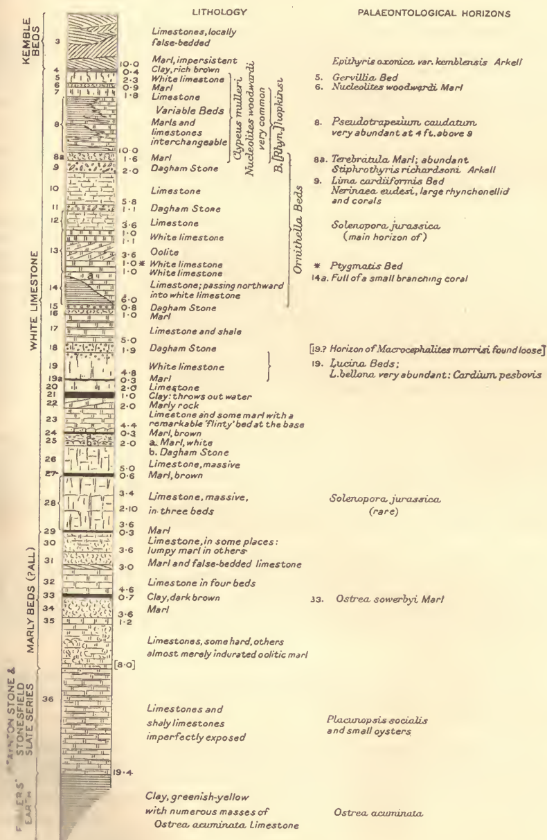
FIG. 2.—Generalized section of the Great Oolite exposed in the railway-cuttings between Cirencester and Chedworth.
